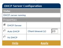
The SpeedTouch<sup>™</sup>570 features a DHCP server which allows the PCs/computers on your local network to automatically obtain an IP address (select DHCP Server). If DHCP is not used on your local network, the SpeedTouch<sup>™</sup>570 DHCP server can be disabled (select No DHCP). The SpeedTouch<sup>™</sup>570 can also search for another DHCP server (select AutoDHCP). If so, it slips into DHCP client mode, if not the SpeedTouch<sup>™</sup>570 becomes DHCP server.
